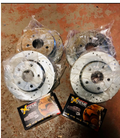
Power stop Z36 brake pads/Drilled and Sotted Rotors
